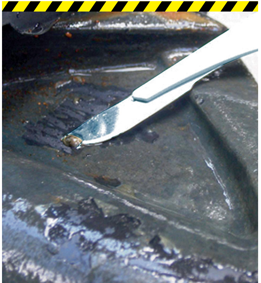
Competitor EPDM wedge after six months of operation - an example of microbiological growth on an improperly formulated rubber compound.
